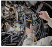
**ULTRA-PORTABLE DESIGN** No need for a separate monitor. Our lightweight, compact design has a builtin, full-color LCD display. All image capture, storage and processing is handled within the standalone unit, and the rechargeable Li-ion batteries delivers up to 4 hours of cordfree run time.
