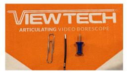
The VJ-3 1.7mm features 2-way articulation, while the non-articulating VJ-4 1.1mm has a flexible insertion tube. Despite their compact design, the 1.7mm and 1.1mm deliver high-resolution imaging, ensuring clear and detailed inspection videos and photos.
