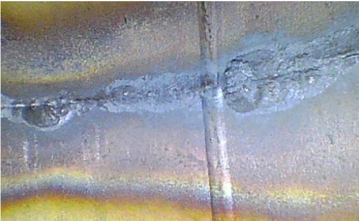
For small ID pipes, the side view camera solves this problem and can provide an excellent, straight-on view of welds in pipes as small as ¾” ID.
