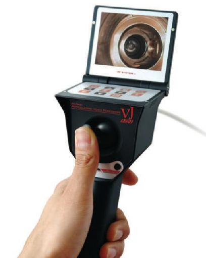
The base imaging unit houses the main PCB, camera articulation controls, video monitor and power supply. *Source: RF System Lab*
