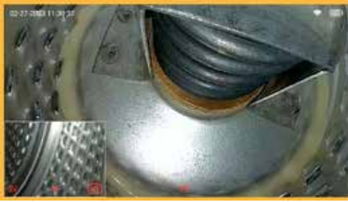
Fig. 8-28 Live Image With the Front View Camera as the Primary Image and the Side View Camera as the Secondary Image
