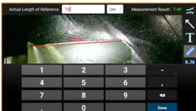
Fig. 8-21 Input the Known Length of Measurement
