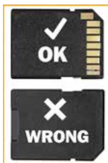
Fig. 8-6 SD card insertion
