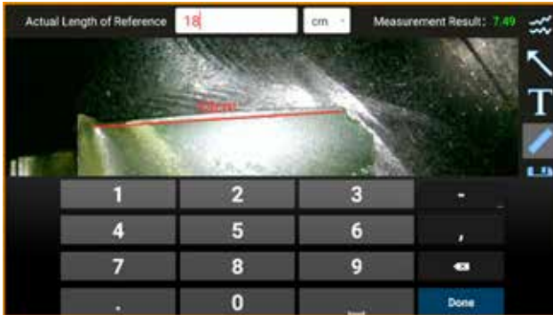
Fig. 8-22 Input the Known Length of Measurement
