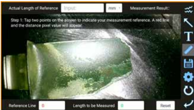
Fig. 8-19 Select an Image to Calculate Reference Measurement
