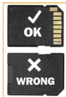
Fig. 8-6 SD card insertion
