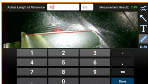
Fig. 8-21 Input the Known Length of Measurement
