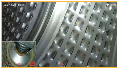
Fig. 8-28 Live Image With the Side View Camera as the Primary Image and the Front View Camera as the Secondary Image
