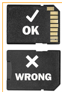
Fig. 8-6 SD card insertion
