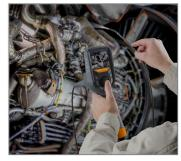
**ULTRA-PORTABLE DESIGN** No need for a separate monitor. Our lightweight, compact design has a builtin, full-color LCD display. All image capture, storage and processing is handled within the standalone unit, and the rechargeable Li-ion battery delivers up to 2.5 hours of cord-free run time.
