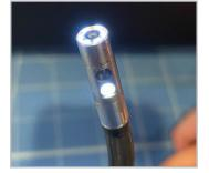
**6.0MM DUAL CAMERA** Available in lengths from 1.5m to 8.0m. The dual camera assists in viewing straight ahead and 90 degrees. Users can switch between the two cameras while keeping the borescope inside the inspection area.
