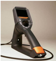
Figure 4: The VJ-3 2.2-mm mechanical articulating video borescope from ViewTech Borescopes.
